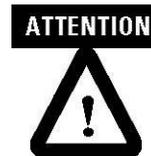
**ATTENTION** Be careful when stripping wires. Wire fragments that fall into a module could cause damage when power is applied. Once wiring is complete, ensure the module is free of all metal fragments.
